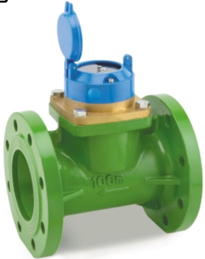
The TURBO-IR uses a multi-blade plastic paddle mounted at the top of the water passage, where disturbance from solids suspended in the water is minimal, permitting accuracy of metering in water containing up to 30% solid debris.
