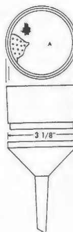
Figure 962.09B—Modified California State Büchner funnel, 2-piece polypropylene plastic, covered with 200-mesh screen, A, heat-sealed to edge of filtering surface
