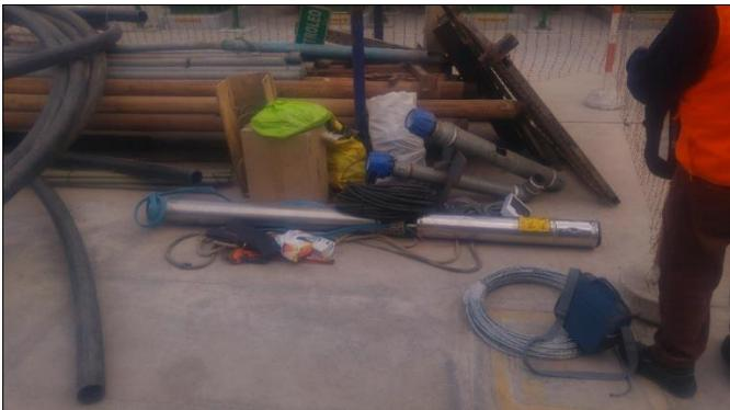
**Figura 13: Electrobomba sumergible Pedrollo (25 HP)**
