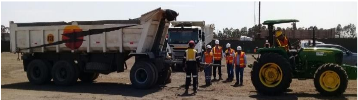
Figura 38: Remolque acople a tractor John Deere Modelo 5075E.
