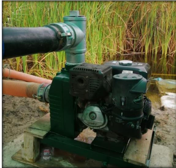
**Figura 6: Motobomba gasolinera.**
