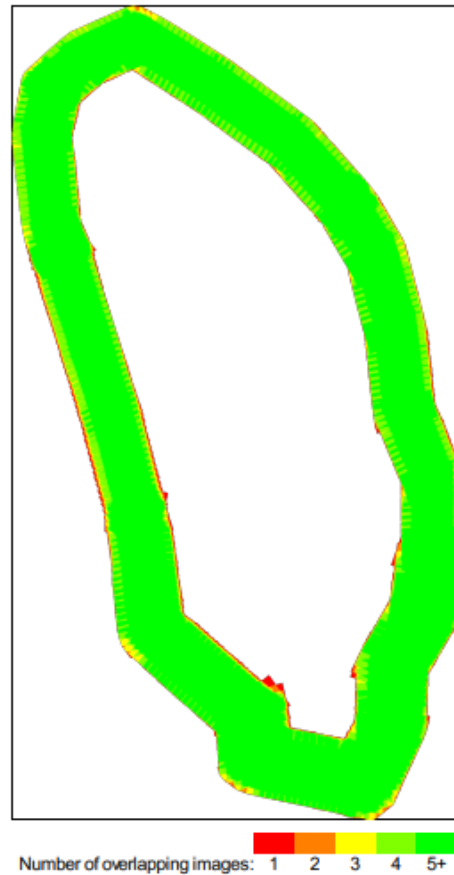
Figure 4: Number of overlapping images computed for each pixel of the orthomosaic. Red and yellow areas indicate low overlap for which poor results may be generated. Green areas indicate an overlap of over 5 images for every pixel. Good quality results will be generated as long as the number of keypoint matches is also sufficient for these areas (see Figure 5 for keypoint matches).
