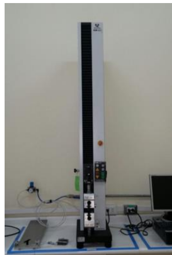
Figura 23: Dinamómetro universal EJA Vantage 225-52215 (Thwing Albert)
